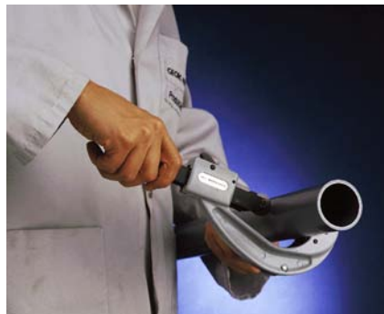
Cutting the pipe to length
