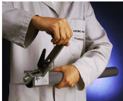
Chamfering the pipe
